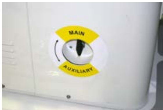
Main/Aux Tank Selector on Engine Box Cover
