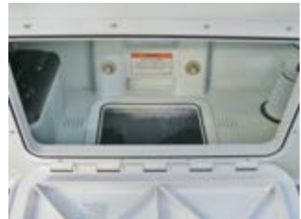
Transom locker and bilge access hatch
