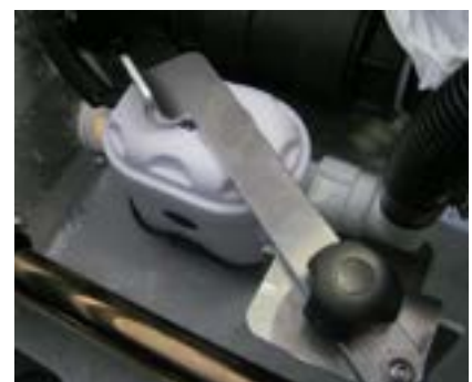
Bilge pump, with locking arm
